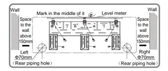
Open a piping hole with the diameter of Φ70 on the selected outlet pipe position. In order to drain smoothly, slant the piping hole on the wall slightly downward to the outdoor side with the gradient of 5-10°.
